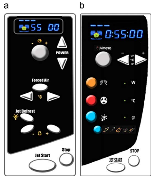
Fig. 8. (a) Commercial (reference) interface and (b) redesigned interface.
